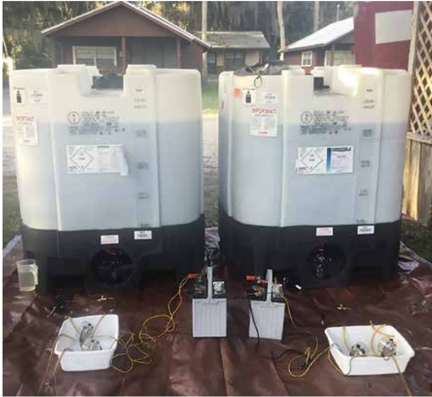
Figure 5. Endothall (Aquathol K, UPL) injection system for the Lake Panasoffkee Outlet River in 2019.
