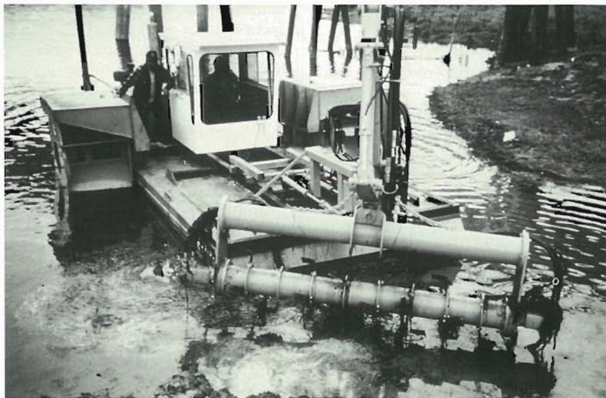
Fig. 3 Barge-mounted rototillers use hydraulic, rotating discs to destroy roots.
