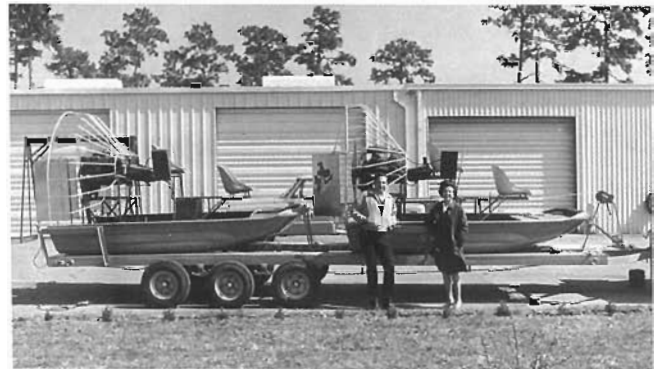
During the fuel shortages of the early 1970s, dual boat-carrying trailers were designed like this one at the Kissimmee Field Station of the SFWMD to conserve energy. Tom Brooks File Photo.
