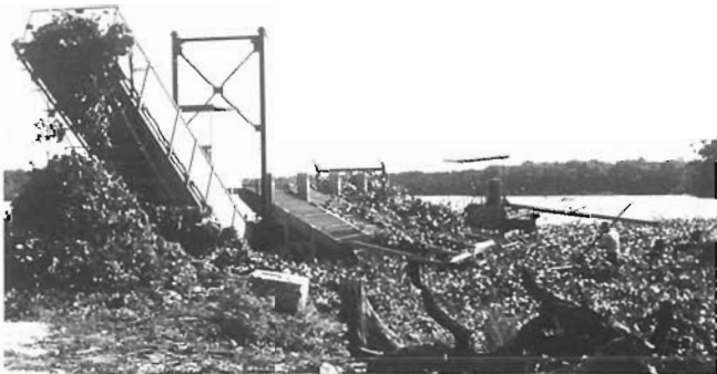
A stationary harvester tested by the DNR for river systems, where plants physically move to the harvester rather than the harvester moving to the plants. The operation was later abandoned. Photo by Clarke Hudson.
