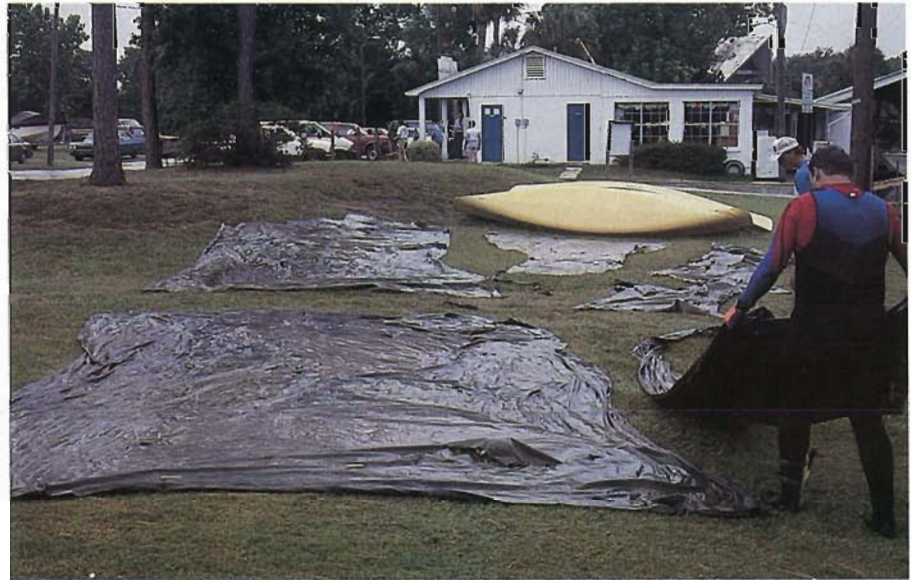
Barrier sheets after 4 months of submersion.
