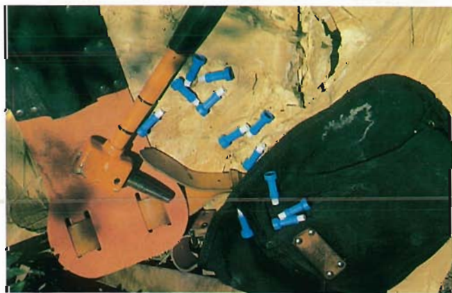
Figure 1. The FIC ® system includes a hammer, leather belt, holster, and a pouch. FISCAN plugs with VELPAR ® herbicide sealed inside are sold separately.
