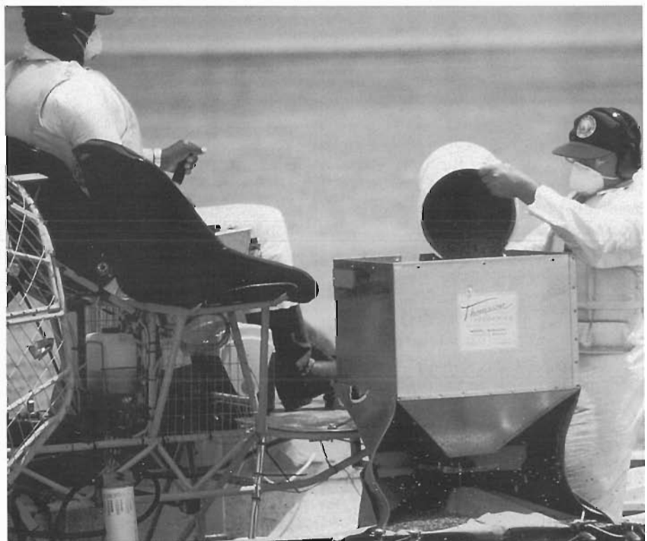
Kissimmee crews apply Sonar® pellets from an airboat
