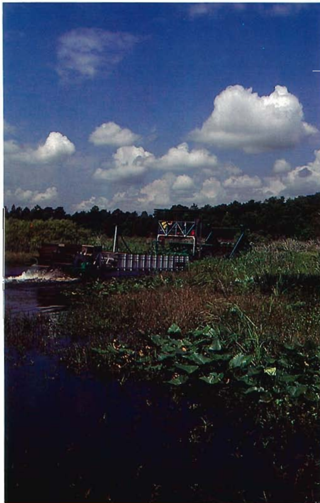
The 70 ft long 15 ton Kelpin 800 harvester removing floating islands on Orange Lake, Alachua County, Florida. photo by Jim Kelly
