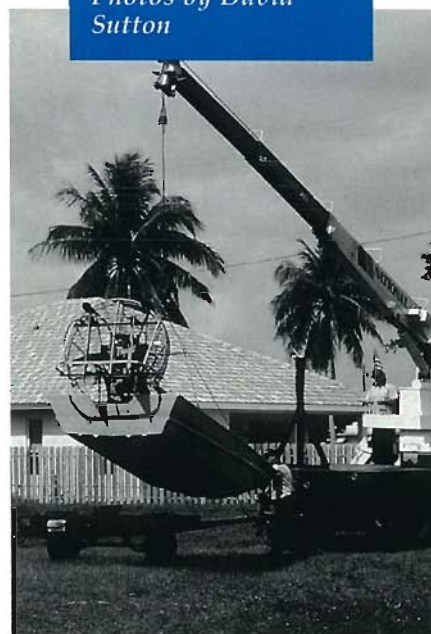
Figure 2. The OPWCD uses a truck-mounted hydraulic lift to set the spray boat in canals when access is limited.
