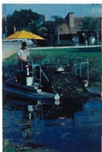
A mechanical harvester is used by the Old Plantation Water Control District to remove heavy infestations of aquatic plants and debris in South Florida. Photo by Dave Sutton
