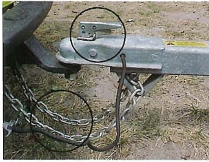
What's wrong with this picture? Install a lock on the coupler lever and receiver hitch to deter thieves and secure the trailer while towing. Also safety chains should be crossed to "catch" the coupler should it become unhitched. Photo by Dave Tarver.
