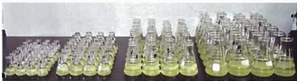
Algal Challenge Test (ACT): A laboratory assessment measuring the effectiveness of different algaecides and rates in the site water containing problem algae.
