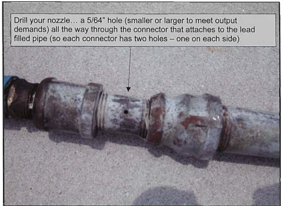
Figure 7. The nozzle for herbicide discharge can be drilled to any appropriate size. Note that the leading edges of the fitting are ground down to minimize snagging on submersed weeds. Photo by Greg Reynolds.
