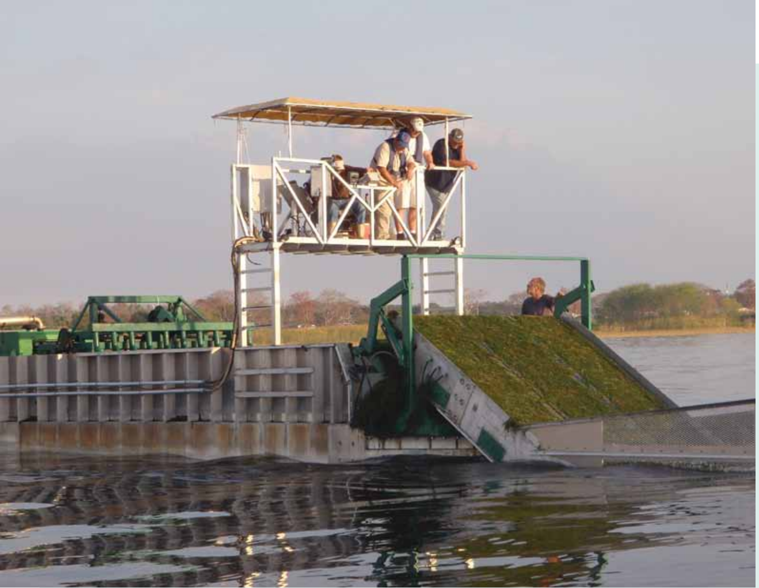
The 70 ft Kelpin Harvester was fitted with GPS navigation and the pickup table extended in order to harvest to a maximum depth of 10 feet, although most of the hydrilla in the Lake Toho site was only 3-6 ft tall in 8-9 ft of water. Photo by Dean Jones.
